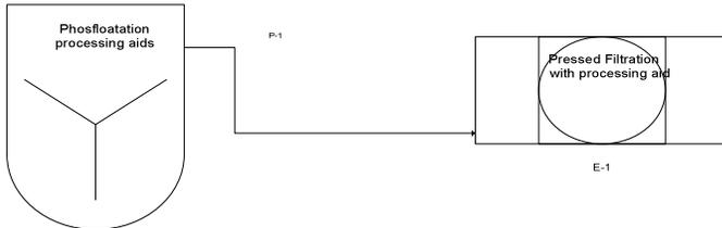
**(II a) Color of input raw sugar exceeds 600 ICU.** In this case, phosphatation process is definitely needed to decolorize the liquor to be less than 275 ICU using various FDA approved purifying aids as shown below. It should be noted that all processing aids used meet US government regulatory requirements.
