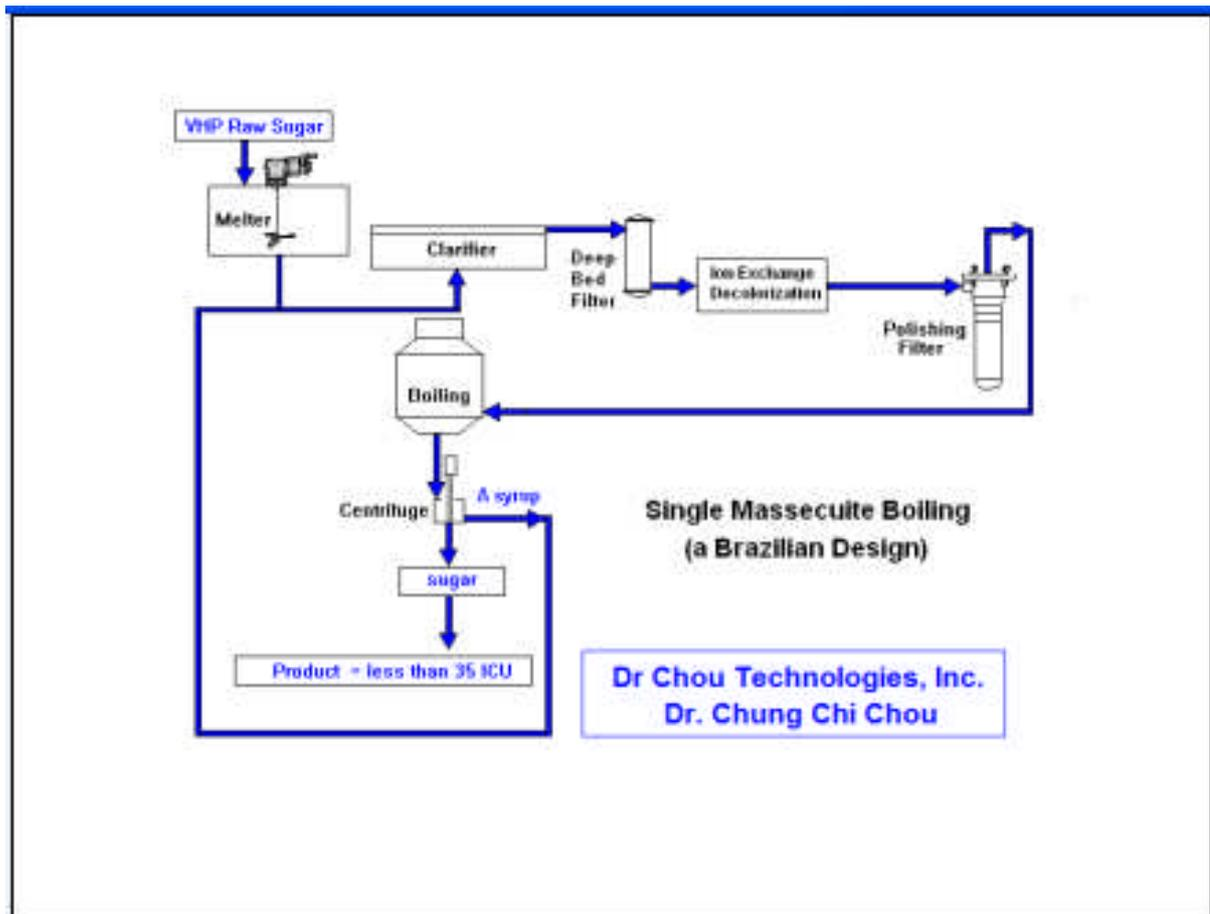
The process only has R1 boiling and recycle all the R1 syrup back to the melter mixing with the melted VHP raw sugar and send it to the clarifier again. Most newer refineries then send the clarified liquor to the deep bed filters to remove any suspended solid over 5 microns, and then to ion exchange resin for final decolorization and crystallization. No filter presses are used
